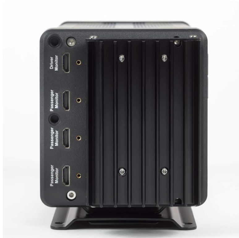
Figure 8 - End panel HDMI connections
